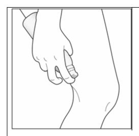
**Step 3:** The foam can be sprayed holding the can in any position except horizontally.
